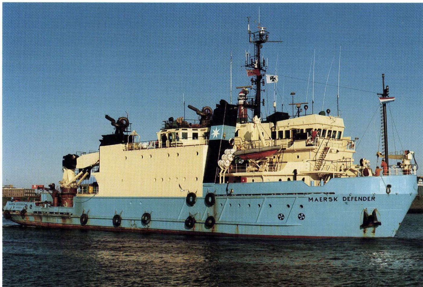
M.s. "MAERSK DEFENDER" is a combined fire-fighting, safety-, rescue- and diving support vessel.
