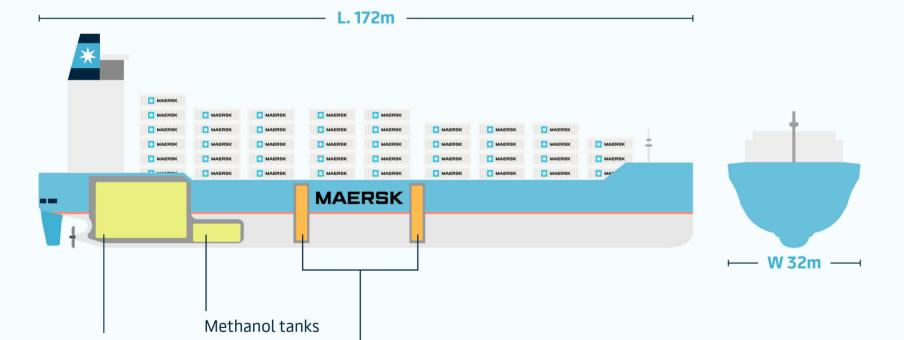
MAN 6G50-LGIM methanol main engine and methanol capable gensets
